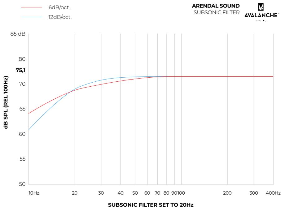
*In this example you can see how the frequencies below 20Hz are affected by adjusting from 6dB/oct. slope to 12dB/oct.*
