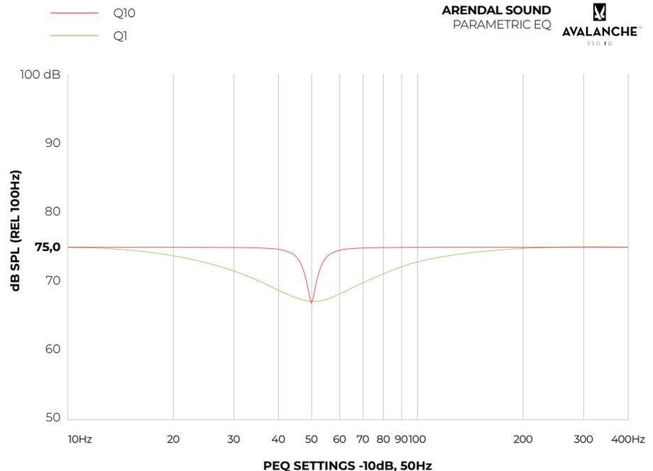
*The graph shows how adjusting the Q settings affects the frequencies above and below the selected frequency you want to adjust. Using a low Q will affect a large bandwidth of frequencies, while a higher Q will only affect areas near the selected frequency.*
